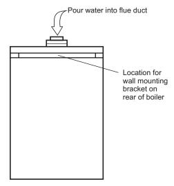
Fig. 4.3 - rear of boiler
