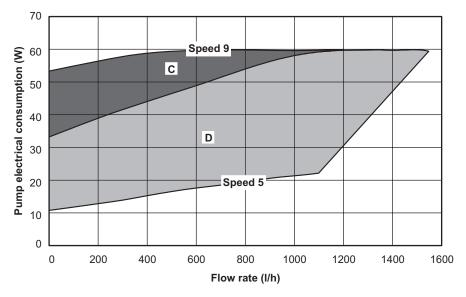
C + D = Pump power consumption with by-pass opened.
