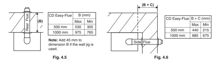
2. Determine the overall length (L) of flue required, (see Fig. 4.7) as follows:-
