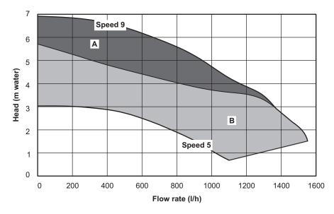
$\label{eq:B} \begin{array}{l} \mathsf{A} + \mathsf{B} = \mathsf{Head} \text{ available to the system with by-pass closed.} \\ \mathsf{B} = \mathsf{Head} \text{ available to the system by-pass opened.} \end{array}$
