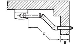
$L = B + E + F + 230 \text{ mm} + (90^{\circ} \text{ bend} = 1.3 \text{ metre})$
