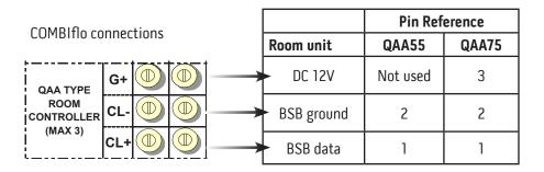
Up to a maximum of three room units can be connected to the same set of QAA connections inside the COMBIflo wiring centre.
