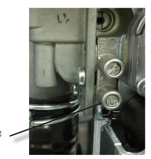
Inlet pressure tapping measurement point
