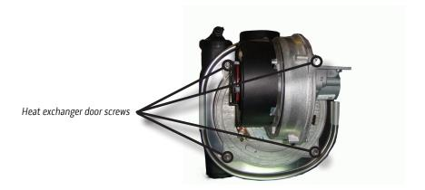
• Remove the whole burner system using the four retaining nuts holding the heat exchanger door to the body.
