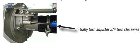
9. Follow the commissioning procedure in section 5.2.2 (points 1 to 36) from page 43 with the exception that the *The CO² combustion figure should now be 10.2% +/- 0.2% for LPG*
