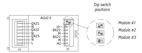
Before use, the purpose of each expansion module must first be defined under engineer login in the configuration menu (parameter lines 6020 - 6022). The following table details the 7 different configuration modes and their pre-configured inputs and outputs:
