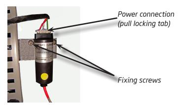
This is located around the rear of the main electronics housing panel. To remove:
