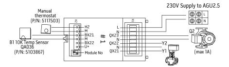
In the above example the setup for "module 1" would be "Heating circuit 1". If the temperature of HC1 needed to be increased, the controls would supply 230V through QX21 (Y1) to open the valve until the temperature rise was detected by the sensor B1. If the temperature of HC1 needed to be decreased the controls would supply 230V through QX22 (Y2) to close the valve until the temperature fall was detected by sensor B1.
