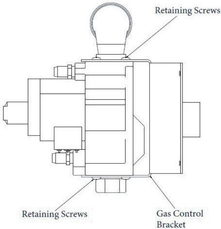
To remove gas control, unscrew four retaining screws at top and bottom of gas control bracket. Also it will be necessary to remove gas fittings at the top of the gas valve and the bottom of the gas valve. It is now possible to slide the gas control valve away from the gas valve retaining bracket.
