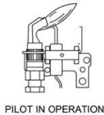
Steel Burner: These models are equipped with self-adjusting air mixture and do not have an adjustable air shutter. At the time of installation and during annual maintenance, a visual check of the pilot and burner flames should be made to determine if they are burning properly. The burner flames should be blue with yellow tips. A blue-orange flame is characteristic of operation on liquefied petroleum (LPG) gas.
