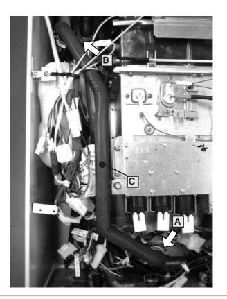
(2) Remove the quick fastener (A) in the right figure and pull the bypass servo (B).
