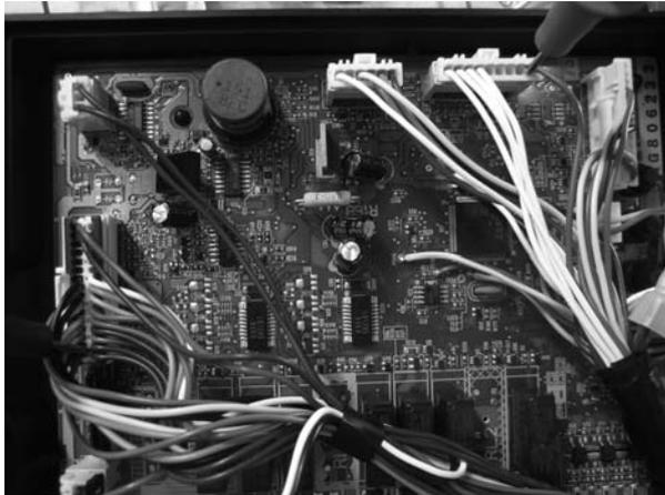
(2) Measure the voltage between Blue 29 of connector 38 and Red 9 of connector 63 on the circuit board.
