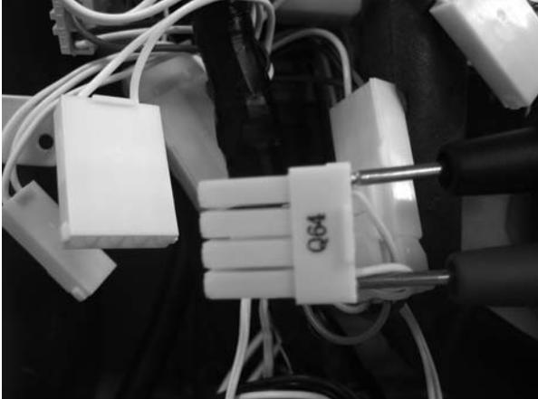
Check the heat exchanger thermistor.
