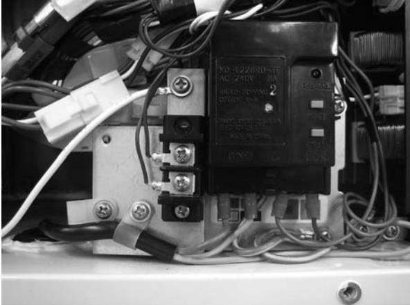
Check the operation of the current leakage safety device.
