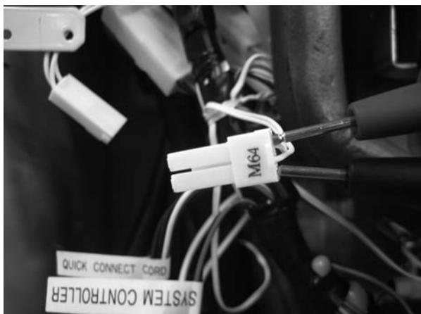
If error display 32 appears, then check the water outlet thermistor.
