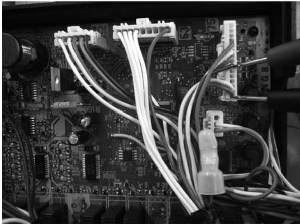
(2) Measure the voltage between Red 1 and Blue 7 of connector 75 on the circuit board.
