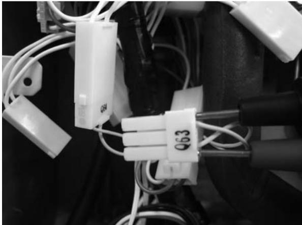
Check the water inlet thermistor.
