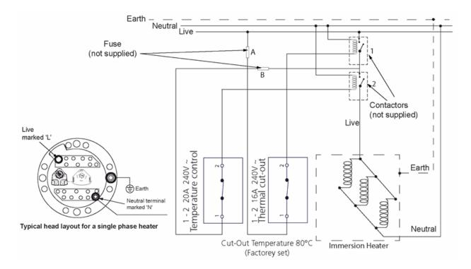
FIGURE 5: Single phase wiring schematic
