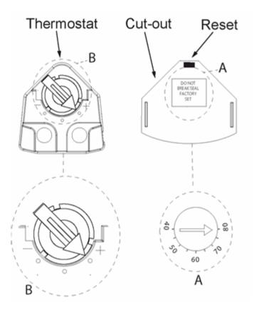
FIGURE 4: Thermostat and thermal cut-out settings
