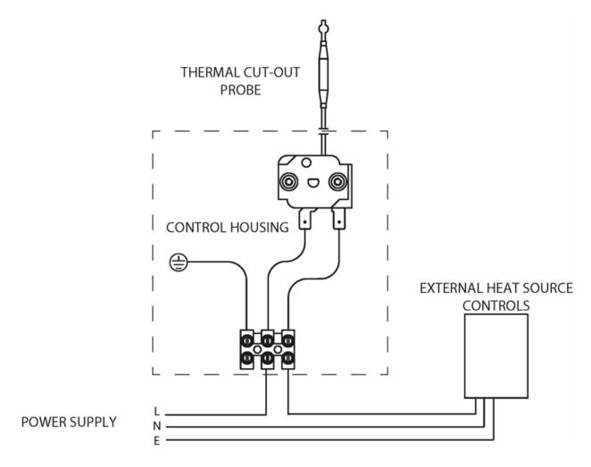
Figure 08: External heat source Thermal Cut-out
