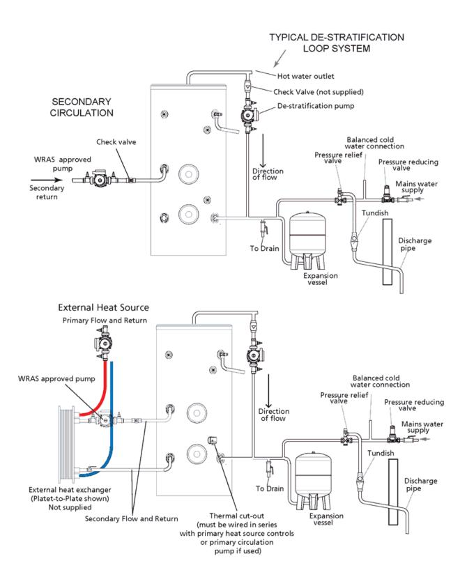
Figure 09: Schematic installations
