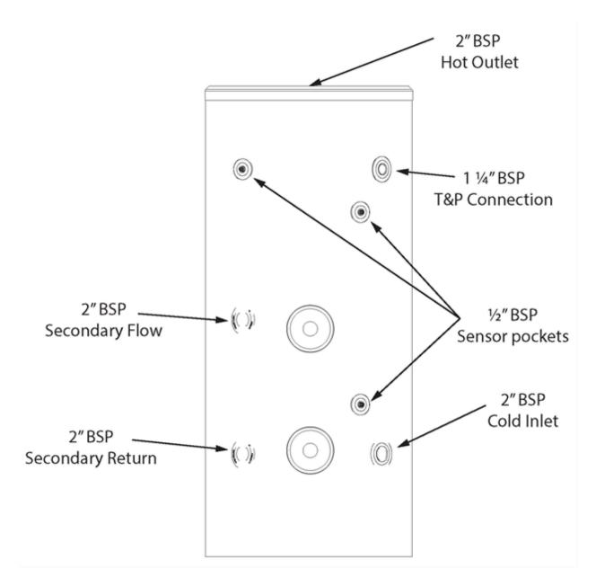
FIGURE 3: Flexistor Connections
