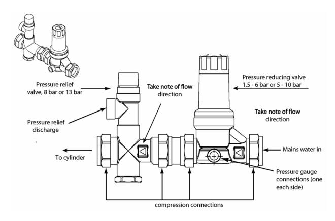
Figure 07: Cold water combination valve (for 400 & 500ltr)
