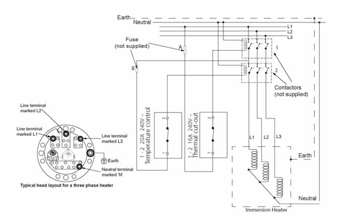
FIGURE 6: 3 phase wiring schematic
