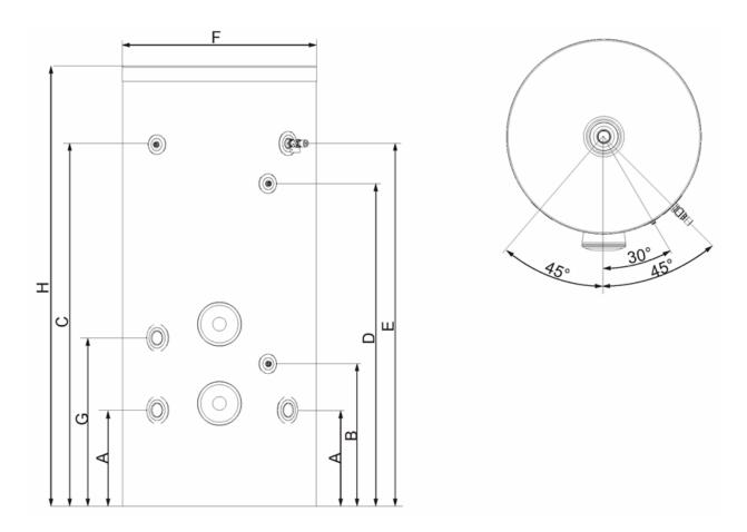
FIGURE 2: Flexistor Dimensions
