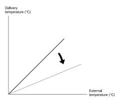
If the following situation occurs: with low external temperatures (e.g. winter, -20°C) the building is adequately heated, but with favourable climatic conditions (e.g. spring, +20°C) it is not sufficiently heated, it is necessary first to choose a lower curve ("F" on the display and then "-") and then turning the heating temperature knob.
