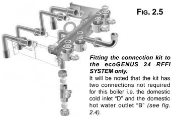
Although the cold water main supply must be connected to the isolation valve for the purpose of operating the filling-loop, the isolation valve is NOT connected to the boiler and should be left in the OFF position.
