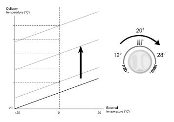
In this manner, temperatures for the water coming out of the boiler are set successively higher, which then influence the room temperature increasing it to the desired settings.
