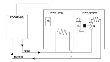
This set-up is simpler and more economical because it does not involve the use of the special relay. The night zone, however, may only be heated during the time periods in which the remote control timer gives consent to the heating of the day zone. Example:
