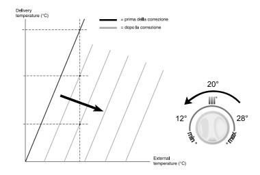
If the room temperature is too cold during the winter (while in spring the temperature is adequate), it is necessary to enter a steeper curve. To do this, press the reset button for 5 seconds and then press it repeatedly until the letter "F" appears (using the "+" and "-" keys). In this manner, the curves may be selected from 1 to 5.
