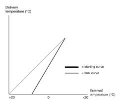
CURVE 4-5: conventional low temperature boilers (cast iron and aluminum radiators, radiant plate systems). Planned temperature 60/45°C.
