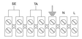
**Note:** The wiring of the Outdoor Sensor (SE) must be done by using 2 x 0.5 mm² cable this guarantees a maximum length of 50 m. The sensor must be positioned at least 2 - 2.5 m above the ground and where possible facing north. The sensor must not be exposed to direct sunlight.
