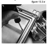
Removing gas air dividing plate figure 13.3.f
