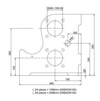
Dimensions low velocity header DN100 until 960kW
