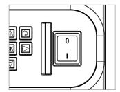
\* Reset only functions in case of an Error or Message. If reset is rapidly pressed over a short period of time, the device will block completely. Only loss of power (unplug) will restart the device completely. Recommendation: First identify the fault by finding the fault code in the fault-code list in the problem-shooting chapter and solve the problem.
