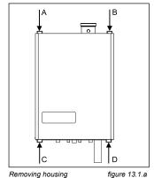
The housing has to be removed in order to carry out maintenance jobs on the boiler. The housing has been secured by 4 quick-lock nuts. First, remove the screws from the quick-locks, open the quick-locks, lift up the housing from below and move it away to the front.
