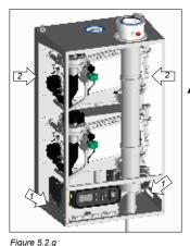
D. Fit a mounting frame on the I-column using 3-x bolt M8x50mm. Refer to figure 5.2.e.
