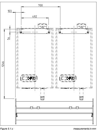
C. Hang the boilers on the suspension brackets.
