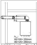
For horizontal sections, the outlet system should always be fitted on an incline (50 mm/m) sloping down towards the appliance so that no condensation water is able to accumulate in the outlet system. The chances of icicles forming on the roof outlet is minimised by causing the condensation water to run back towards the appliance. In the case of horizontal outlets the inlet system should be fitted on an incline sloping down towards the outside to prevent rainwater from coming in.
