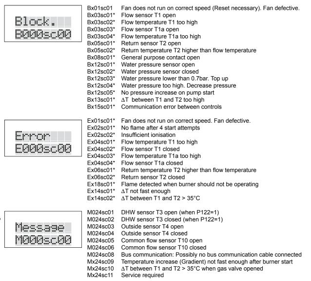
\* When this code is shown with an M instead of a B or E then a reset with the reset button is possible.
