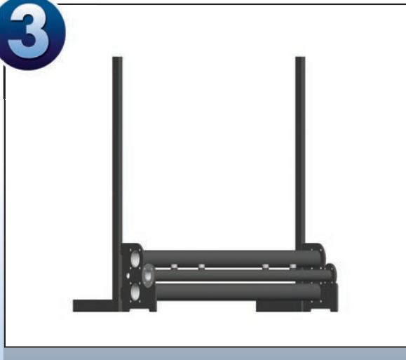
Step 3: Fit 'L' or 'I' support frames
