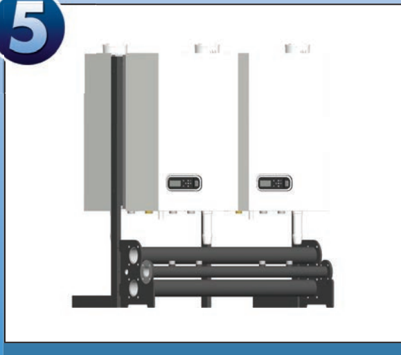
Step 5: Hang boilers
