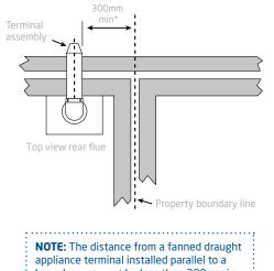
appliance terminal installed parallel to a boundary may not be less than 300mm in accordance with the diagram.
