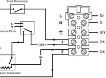
IMPORTANT: If an integral timer is fitted to the boiler an external frost thermostat wired as shown will not operate correctly. Only external timers may be used in such installations, as in the diagram.
