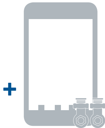
Pre-plumbing jig (including isolation valves)
