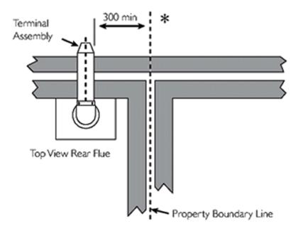
st Reduction to the boundary is possible down to 25mm but flue deflector part no. 5111068 must be used.
