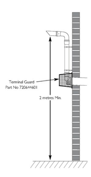
The outlet of the PDK **MUST** be at least 2 metres above ground or balcony level. If necessary additional 60  $\emptyset$  extensions should be used to achieve this.
