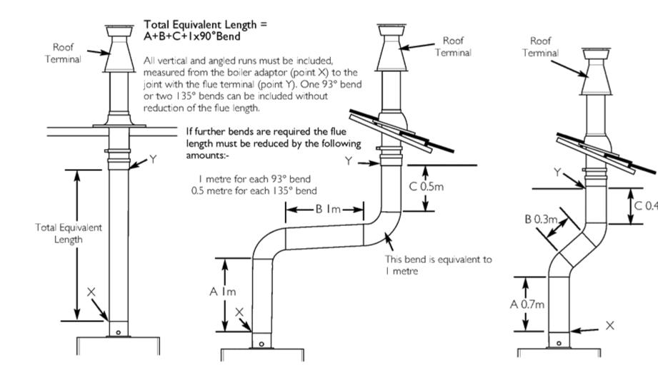
The MAXIMUM total equivalent length is stated in the Installation & Servicing Instructions supplied with each boiler.
