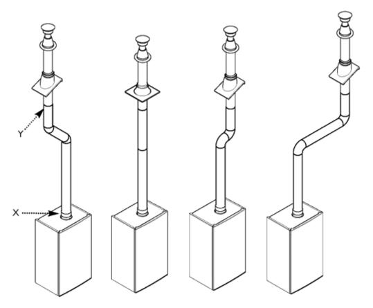
The adaptor shown is available separately for vertical flue applications. (It is included with the 80/125 Horizontal Flue Kit).
