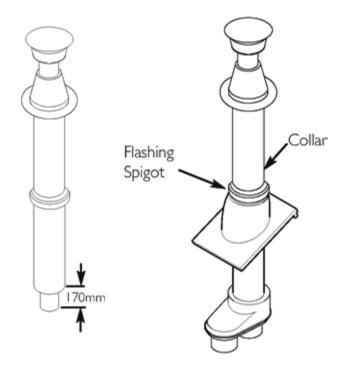
Cut air duct to leave 170mm of exhaust duct protruding page 11
