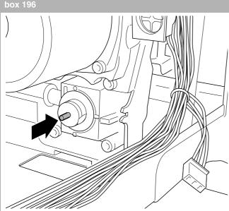
• Check to ensure that the drive mechanism of the 3-way valve is running smoothly. This is done by gradually pushing the spring fully home by hand and allowing the spring to return gradually to its home position.
