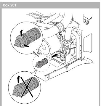
• Fit the new drive mechanism on the internal 3-way valve. Ensure that the flat side faces upwards.
