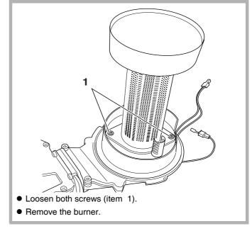
• Fit the new burner to the gas/air unit. Note that a new seal must be fitted between the burner and gas/air unit.
