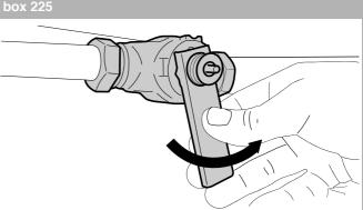
Remove the drive mechanism of the Buderus 24V AC external 3-way valve using the wrench supplied with the drive mechanism.
