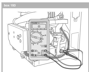
• Check the power supply cable of the 3-way valve for internal short circuits. The level of electrical resistance, measured between two wires chosen at random, must be infinitely high.
