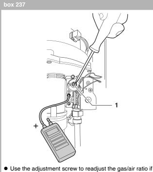
Use the adjustment screw to readjust the gas/air ration necessary (item 1).
