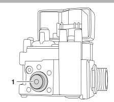
• Fit the gas valve to the new fan. When doing so, ensure that the gas injector (item 1) is correctly fitted.
