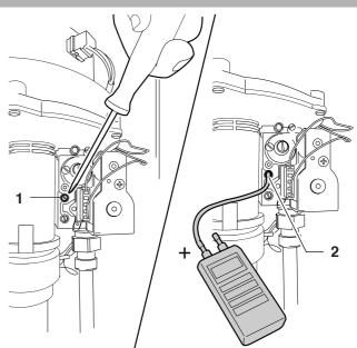
Reset the digital pressure gauge to zero.
