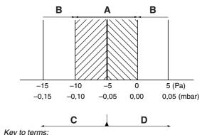
A = correct; B = false; C = turn anticlockwise;D = turn clockwise
