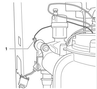
Check to ensure that the earth (ground) lead of the ionisation circuit (item 1) has been correctly fitted.
