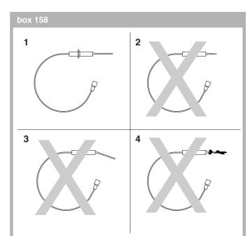
Check the ionisation electrode for signs of wear (item 2), damage (item 3) or soiling (item 4).
