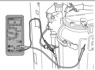
• Take an earth (ground) reading check whether there is a possible short circuit between the cable of the ionisation electrode and earth (ground). The electrical resistance between the ionisation electrode cable and earth (ground) must be infinitely high.
