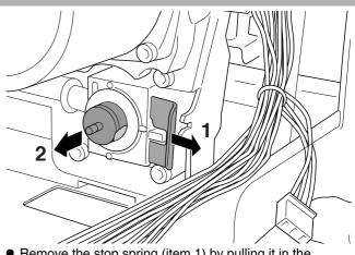
• Remove the stop spring (item 1) by pulling it in the direction of the arrow.
