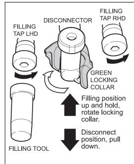
If the Central Heating (C.H.) pressure falls below 0.4 bar the display will flash the current pressure and the boiler will not operate. To increase the pressure the CH circuit requires "Topping up". Push the disconnector up then turn the green locking collar to lock the disconnector in the filling position. Fully open the
