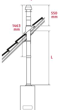
L = Flue length, measured from the top of the boiler to the underside of the roof flashing Maximum flue length is 10m plus external vertical roof terminal.
