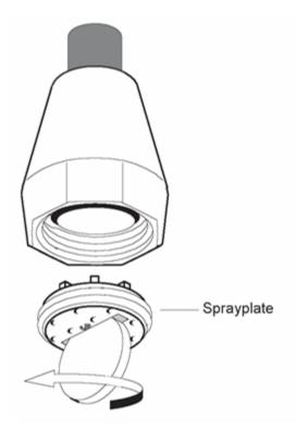
To remove sprayplate unscrew anticlockwise using a coin.
