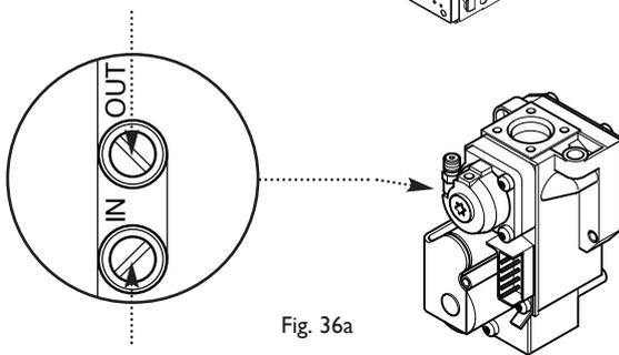
Inlet Gas Pressure Test Point
