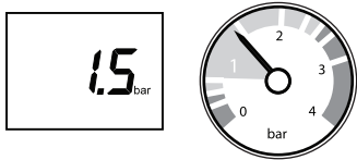
Fig.51 Restore water pressure
