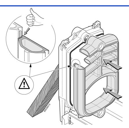
Check the positioning of the thermocord.
