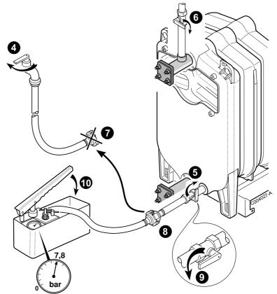
Maintain pressure for at least 10 minutes. Any drop in pressure indicates a leakage in the boiler body
