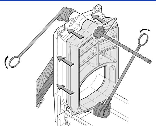
Caution: Do not overtighten. Correct tightening is achieved when the cast iron sections come into contact.
