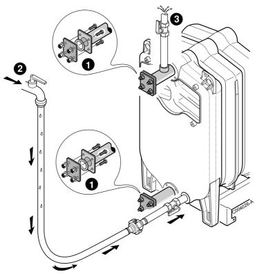
Ensure that all the air in the boiler is vented to avoid any bursting of the body.
