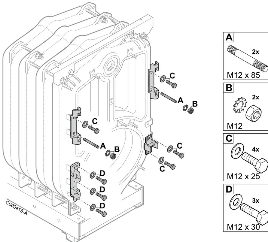
**i** Fit the hinge on the door of the combustion chamber (boiler body accessories package) to the left or right depending on which way you wish to open it.
