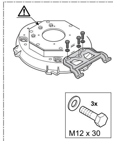
**!** Leave the 3 screws HM12x30 and the 3 washers L12 in place on the combustion chamber door on the side opposite to the added hinge.
