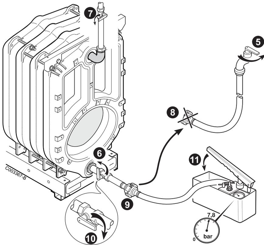
Maintain pressure for at least 10 minutes. Any drop in pressure indicates a leakage in the boiler body.
