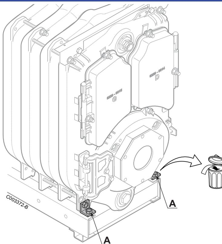
Boilers supplied with an assembled body: Unscrew the screws and remove the A brackets.
