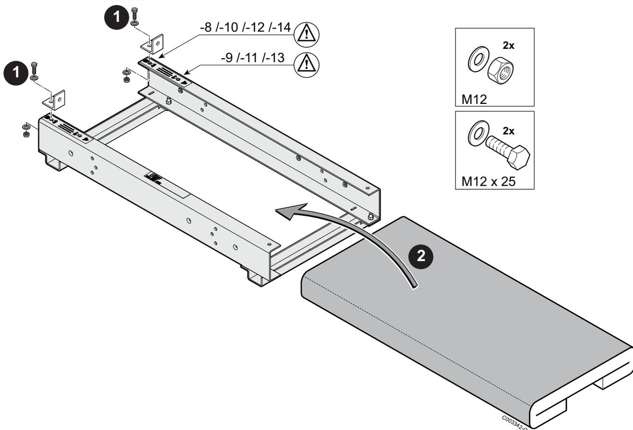
**⚠** Use the holes corresponding to the number of the boiler's elements, following the indication on the frame.
