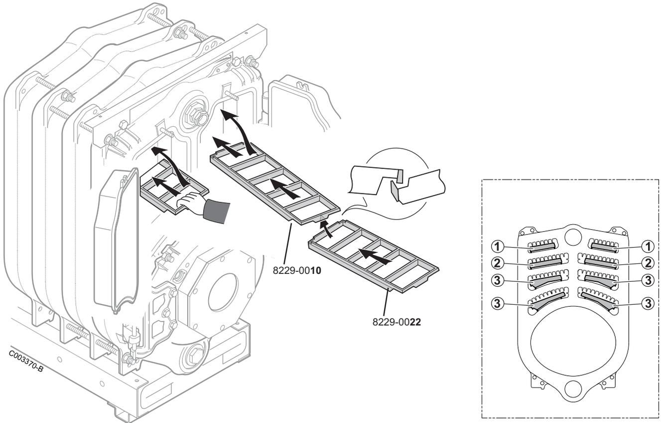
**i** The 8-figure part number of the baffle plate is cast in the metal. **!** Insert the baffle plates flush with the front element.
