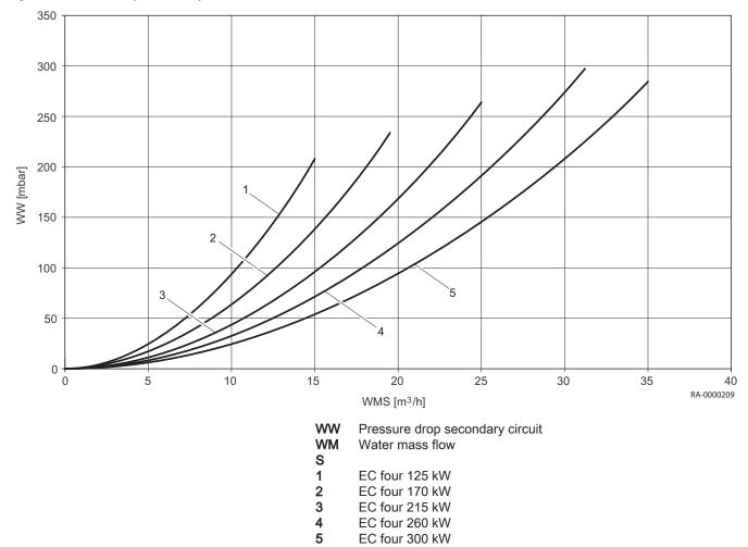
Fig.1 Pressure drop secondary circuit
