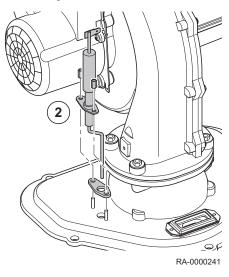
2. Remove nuts and pull out the ionization electrode with the seal
