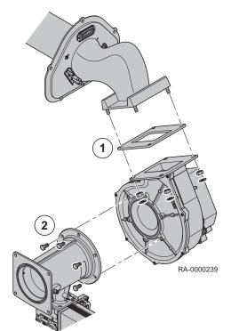
Reinstall the siphon 5. Replace the cover of the exhaust collection pan 6. Note Use a new seal when installing the cover. 7. Reinstall the burner For more information, see Removing the burner, page 132
