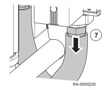
7. Release gas connection hose from the gas valve
