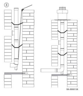
The ducts for exhaust gas facilities must not have any openings other than the necessary cleaning and inspection ports as well as openings for back ventilation of the exhaust gas pipe.
