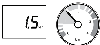
Fig.46 Restore water pressure
