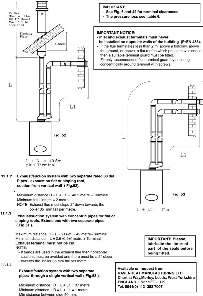
**IMPORTANT:** Please, lubricate the internal part of the seals before being fitted.
