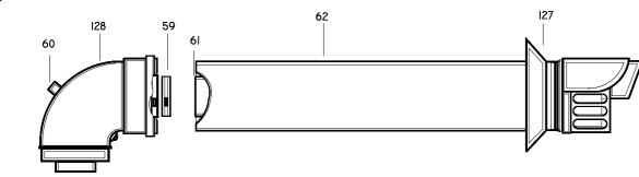
**FLUE EXTENSION BOX CONTAINING** (Fig. 11): 1000 mm flue extension duct as an extra cost only when requested for side and vertical flue applications.
