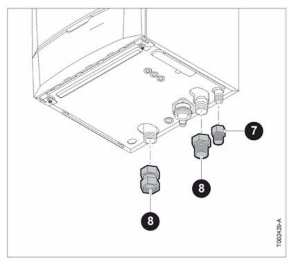
2 40 Nm 3 30 Nm 4 40 Nm 5 • Tighten hand tight. then tighten by a further 3/4 turns. 6 7 30 Nm 8 50 Nm 9 15 Nm 10 15 Nm 11 35 Nm 12 35 Nm
