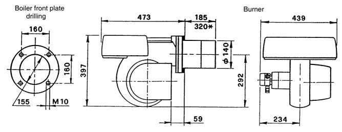
\* Length available with special blast tube to be separately required.
