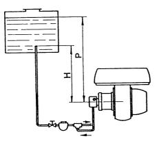
The dimension P should not exceed 10 m, to avoid breakage of pump seals.
