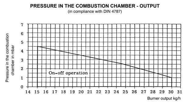
The burner is drawn for on-off operation and high-low operation. Minimum firing-rate at on-off operation is 15 kg/h (two nozzles) and 9 kg/h (one nozzle) with high-low operation.
