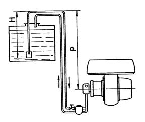
The dimension P should not exceed 10 m, to avoid breakage of pump seals.
