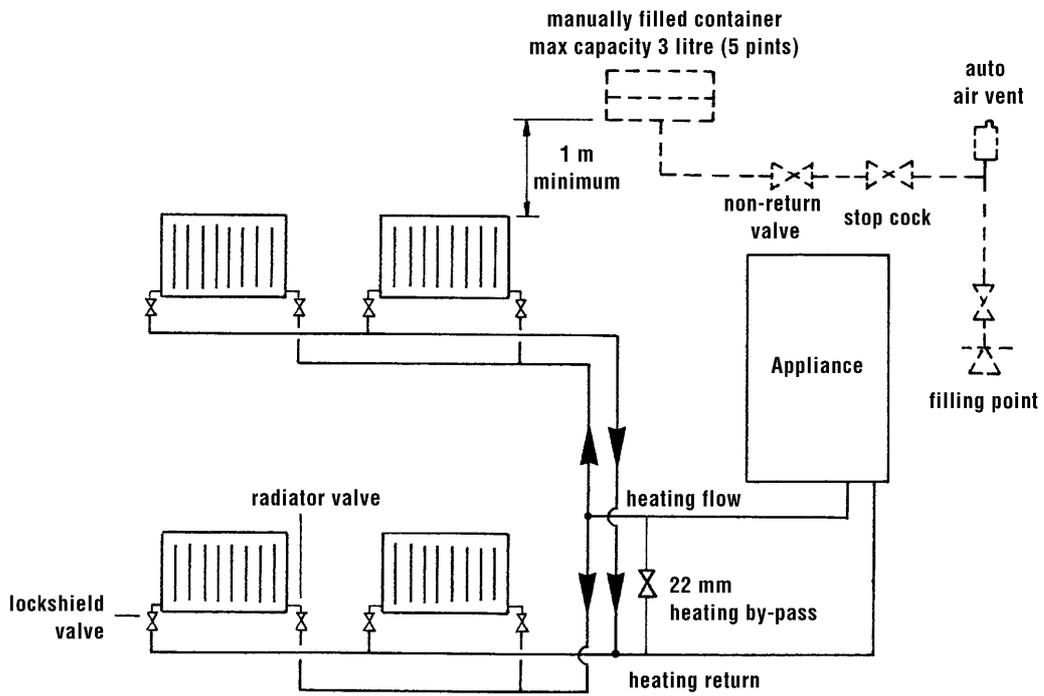
NOTE: A drain cock should be installed at the lowest point of the heating circuit and beneath the appliance.
