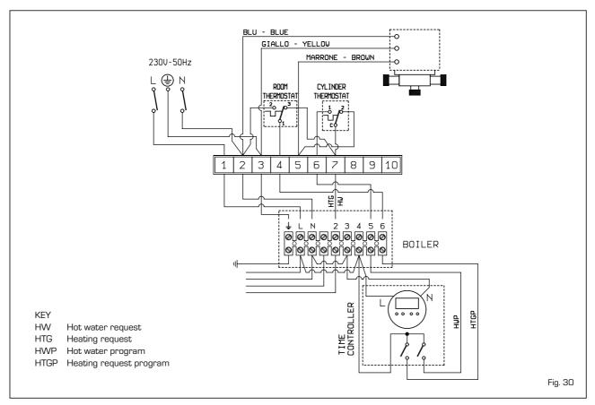
7.6 SYSTEM USING TWO ZONE VALVES
