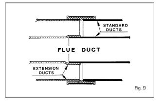
Push an air duct in to the clamp. Join the air ducts (larger ducts) and tighten the screws an the clamp to connect them.
