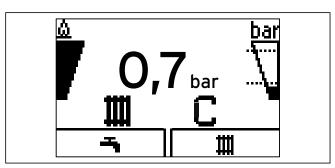
5.2 Display of the filling pressure for the heating installation is too low
