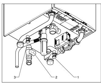
4.6 Opening the isolator devices (shown using the example of service valves)
