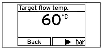
4.10 Setting the heating flow temperature
