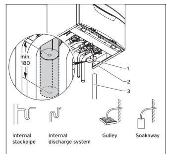
The product is equipped with a condensate trap (2). (The filling height is 145 mm). The condensate trap collects the condensate that has formed in a vessel with a capacity of approximately 200 ml, and intermittently releases the contents into the discharge pipe. This minimises the risk of the discharge pipe freezing.
