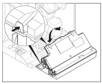
Open the electronics box as shown in the illustration.
