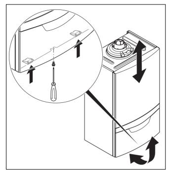
Remove the front casing as shown in the illustration.
