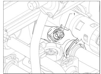
Regulate the pressure using the adjusting screw (1).
