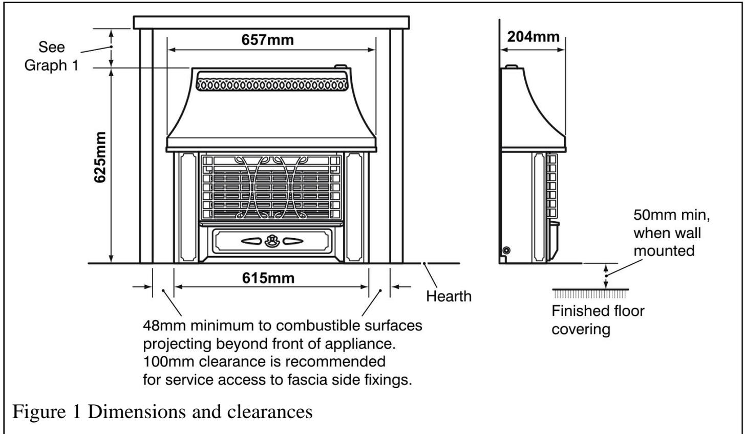
Figure 1 Dimensions and clearances
