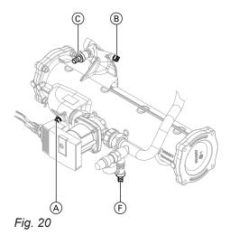
**1.** Close shut-off valve (A) on the heating water side.
