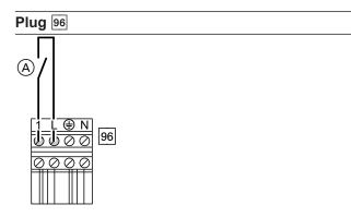
A Floating contact (when connecting, remove jumper between L and 1)
