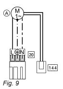
Insert plug 144 (0 - 10 V connection) at X4.
