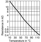
Fig. 46 Sensor type: NTC 10 kΩ
