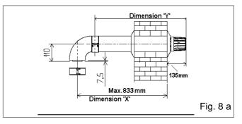
Seal the flue assembly to the wall using cement or a suitable alternative that will provide satisfactory weatherproofing. The exterior trim can now be fitted.
