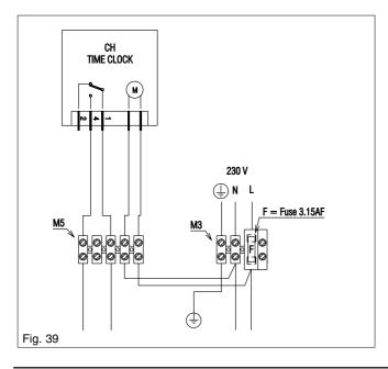
Isolate the appliance from the electrical supply and remove the clock blanking disc from the clock aperture on the boiler. Keep the screws safe, as they will be required to secure the programmer to the aperture.
