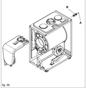
6.20.1 DHW FLOW RESTRICTOR (Fig. 35A)
