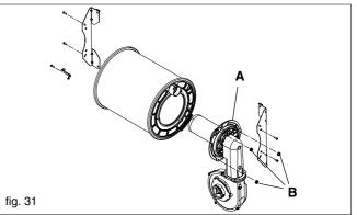
Fig. 31: To remove the fan burner assembly (A) locate and remove the 3 external nuts (B). Replace in the reverse order. Ensure all seals are in good condition, taking care to ensure they are replaced correctly.
