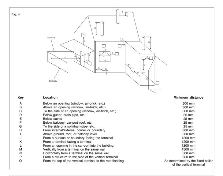
This appliance must be installed by a competent person in accordance with the Gas Safety (Installation & Use) Regulations.
