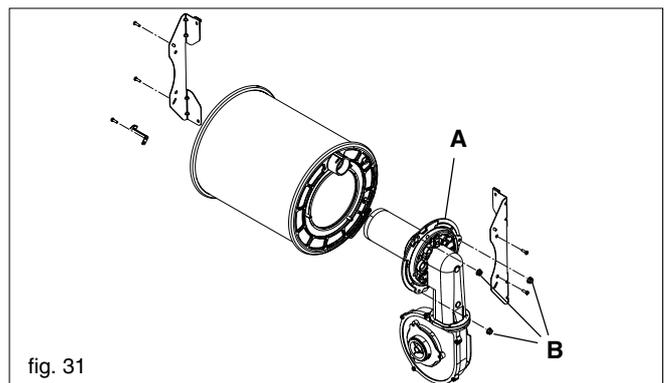
**Fig. 31:** To remove the fan burner assembly (A) locate and remove the 3 external nuts (B). Replace in the reverse order. Ensure all seals are in good condition, taking care to ensure they are replaced correctly.
