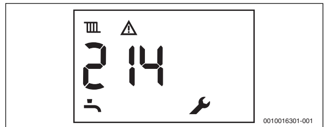
Fig. 8 Example of a fault code
