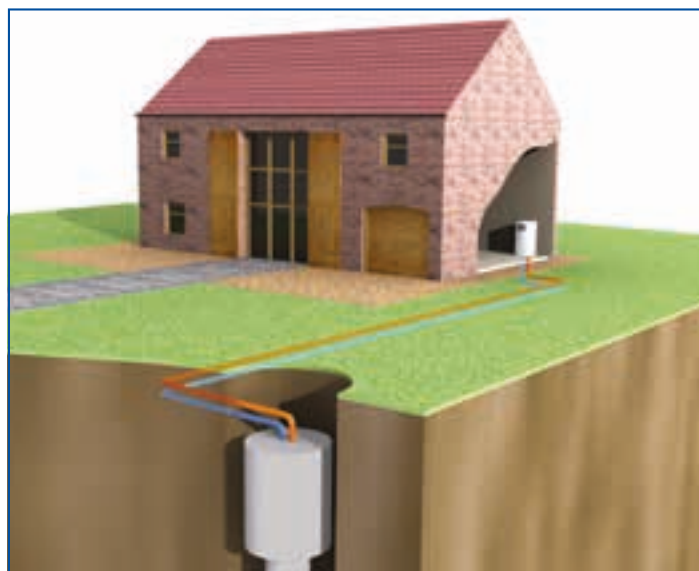
Example of bore hole collector system
